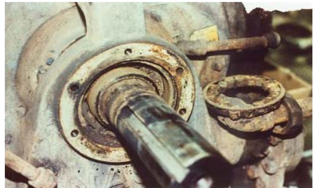
**Most bearing failures are not caused by a bearing manufacturing defect. Bearing failure mode is usually caused by lubricant breakdown or above-normal bearing loads.**
