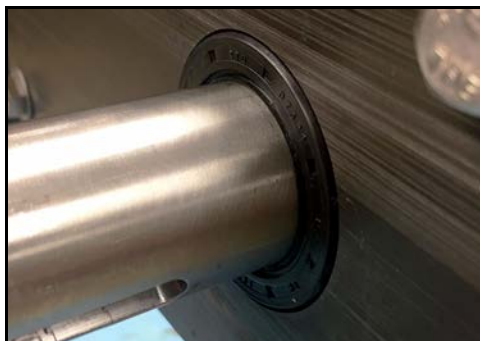
Figure 227 - Oil seal installed
