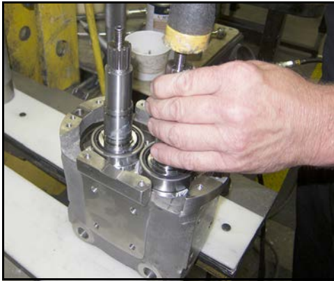
Figure 180 - Tap shafts to center in bores
