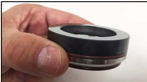
Figure 96 - Seal seat installed on seal cap
