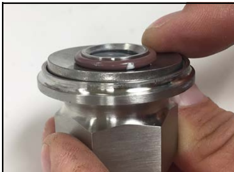
Figure 109 - Belleville washer installed
