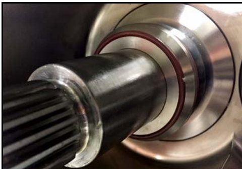
Figure 98 - Seal cap installed on shaft
