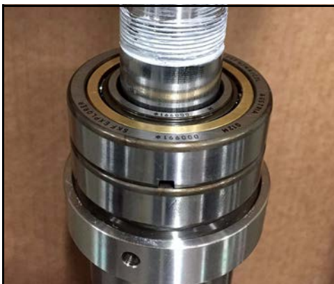
Figure 162 - Second bearing installed
