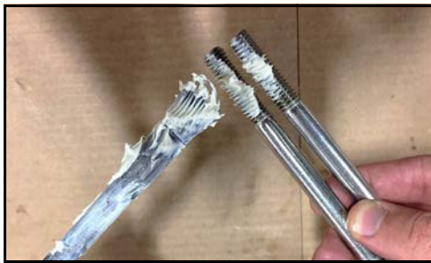
Figure 83 - Apply anti-seize to threads
