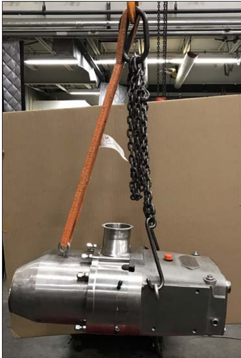
Figure 3 - Lifting location - 130, 220-UTS
