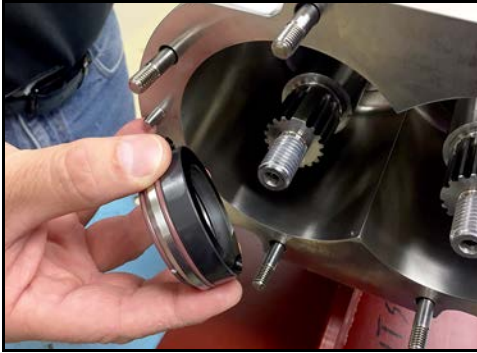
Figure 37 - Remove seal cap assembly
