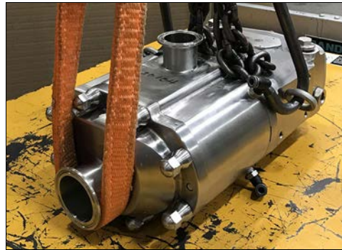
Figure 2 - Lifting location detail - 015, 030-UTS
