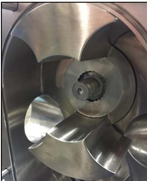
**Figure 178 - Rotor installed**
