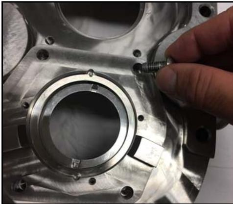
**Figure 88 - Seal housing bolts**
