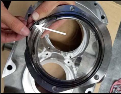
**Figure 77 - Remove seal housing O-ring**
