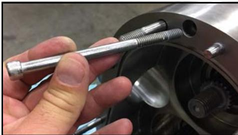
**Figure 42 - Remove body retaining screws**
