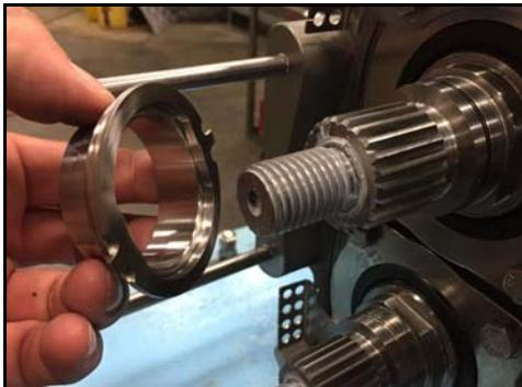
**Figure 68 - Remove adjusting ring**
