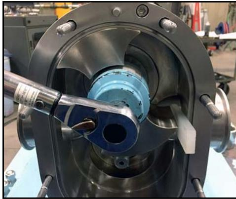
**Figure 35 - Remove Rotor Nut**
