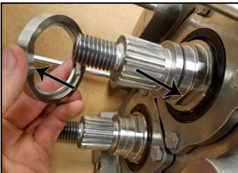
**Figure 162 - Install seal seat**
