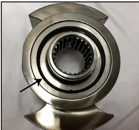
**Figure 136 - Seal O-ring installed**
