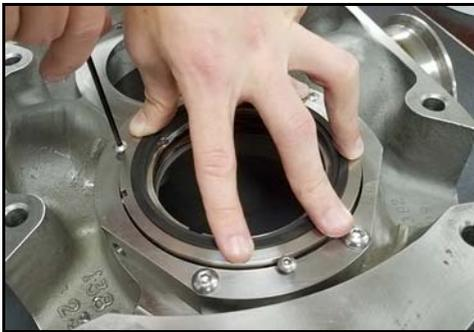
**Figure 117 - Install seal retaining bolts**
