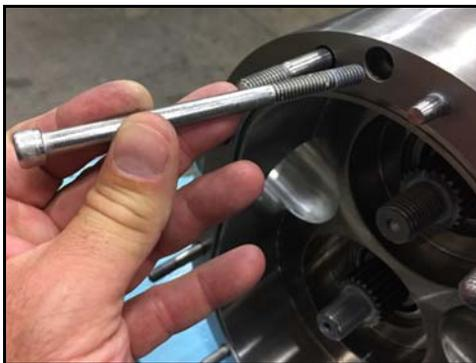
**Figure 129 - Install body retaining screws**
