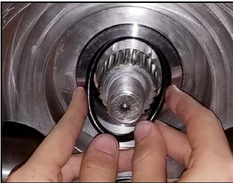
**Figure 168 - Install seal O-ring**
