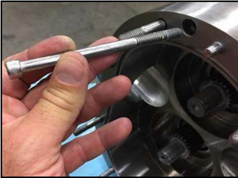
**Figure 167 - Install body retaining screws**
