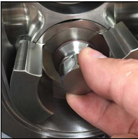
Figure 181 - Install rotor nut
