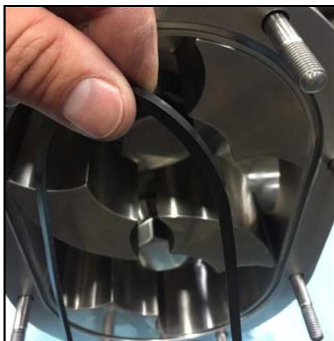
**Figure 184 - Install cover gasket**
