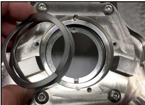
**Figure 72 - Remove wave spring**
