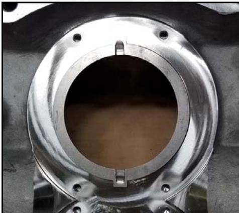
**Figure 61 - Drive ring installed**
