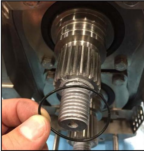
**Figure 119 - Install O-ring**
