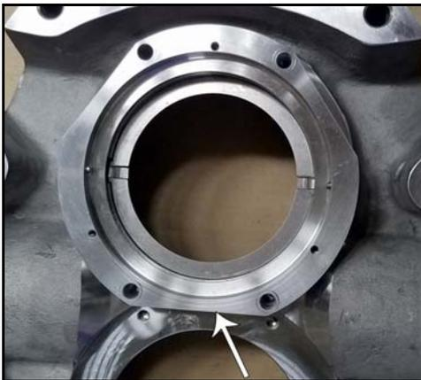
**Figure 111 - Seal housing in place**
