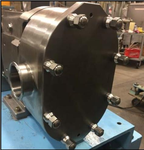
**Figure 188 - Cover installed**
