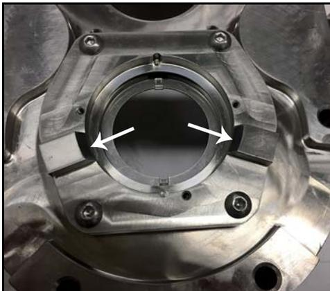
**Figure 89 - Seal housing installed**
