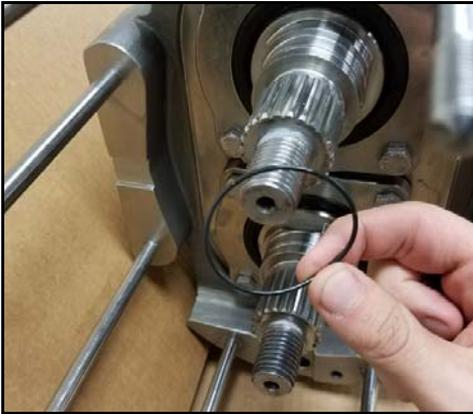
**Figure 160 - Lubricate and install O-ring**
