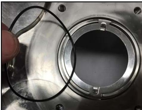
**Figure 76 - Remove seal housing O-ring**
