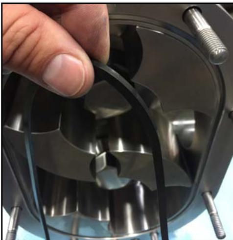
**Figure 34 - Remove cover gasket**
