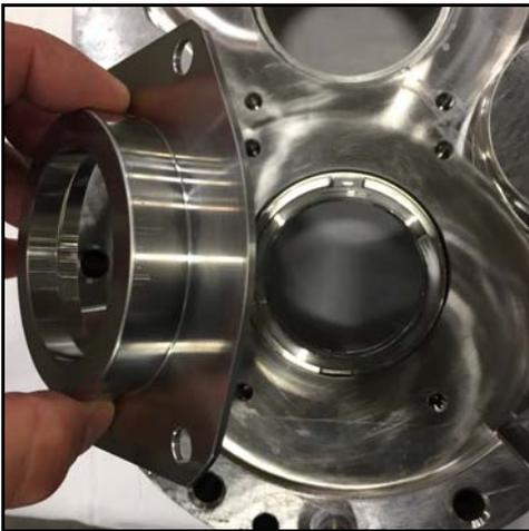
**Figure 45 - Remove seal housing**
