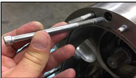
**Figure 147 - Remove body retaining screws**
