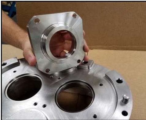
**Figure 150 - Remove seal housing**
