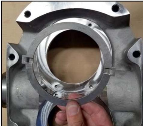
**Figure 107 - Install drive ring**
