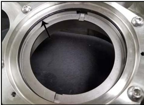
**Figure 114 - Seal O-ring location**
