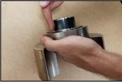
Figure 174 - Lubricate seal sleeve
