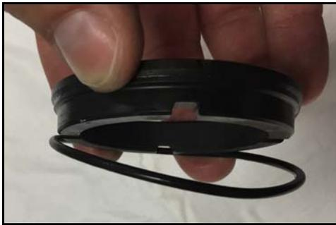
**Figure 41 - Stationary Seal O-ring**
