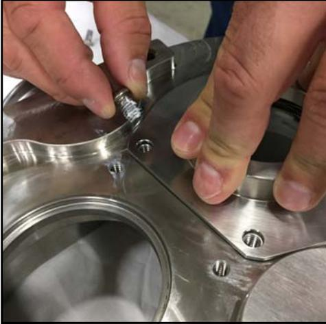
**Figure 44 - Remove seal housing bolts**
