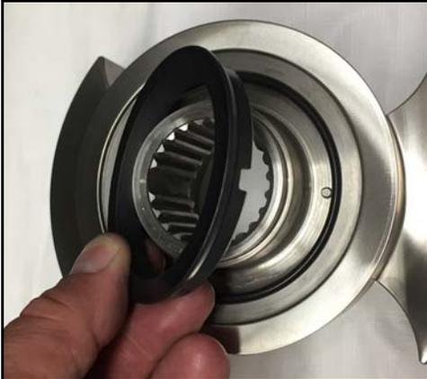
*Figure 38 - Remove rotary seal*
