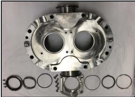
**Figure 80 - Double Mechanical Seal (040-U3 shown)**
