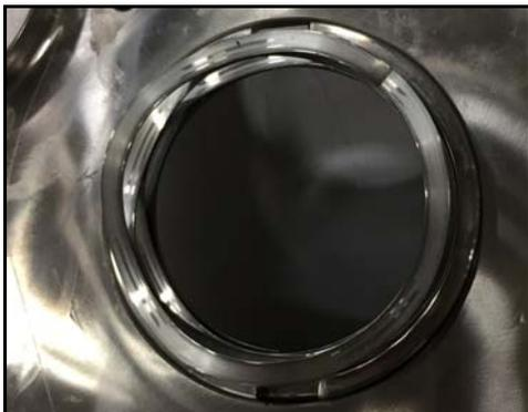
**Figure 56 - Wave spring installed**
