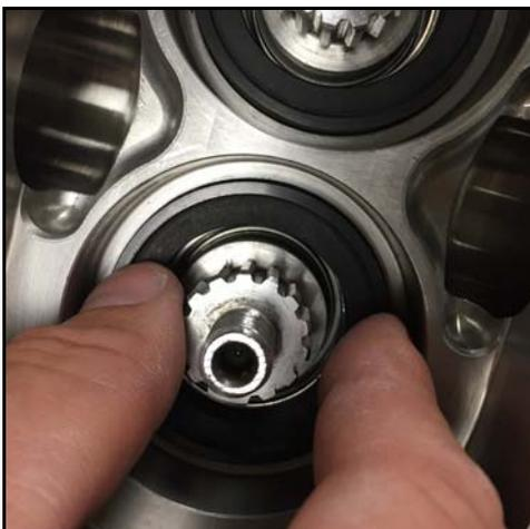
**Figure 133 - Push on stationary seal**
