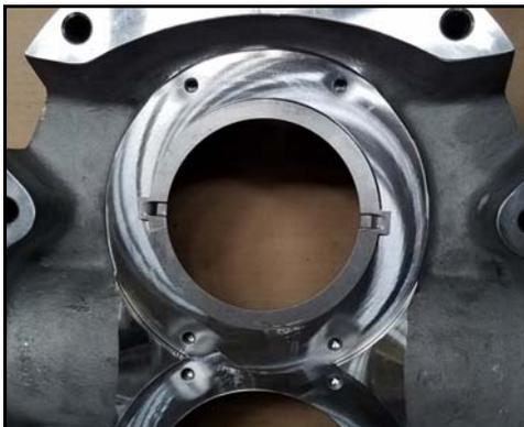
**Figure 108 - Drive ring installed**
