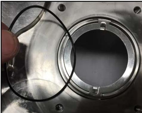
**Figure 85 - Install seal housing O-ring**
