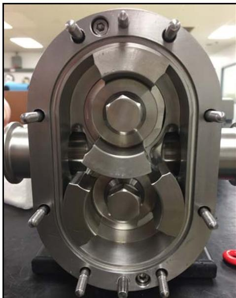
**Figure 183 - Rotors installed**
