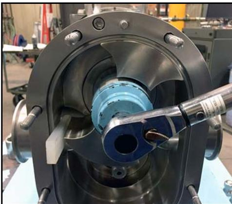
Figure 182 - Torque rotor nut
