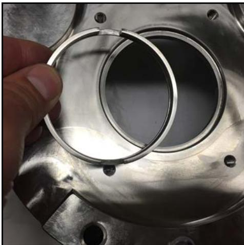
**Figure 81 - Install shaft ring**
