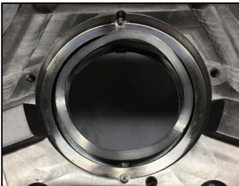
**Figure 93 - Wave spring installed**
