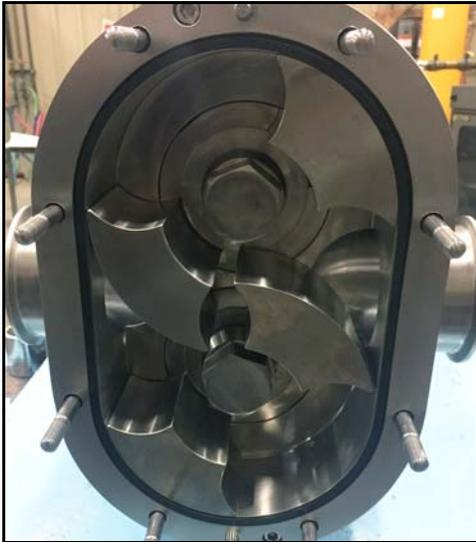
**Figure 185 - Cover gasket installed**
