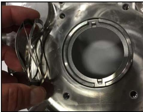
**Figure 55 - Install wave spring**
