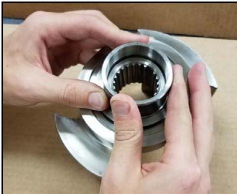
**Figure 172 - Press sleeve into place**
