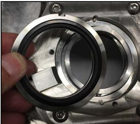
**Figure 71 - Remove stationary seal**
