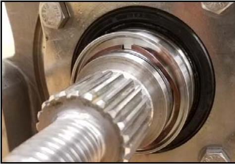
**Figure 164 - Install wave spring**
