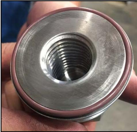
Figure 180 - O-ring installed
