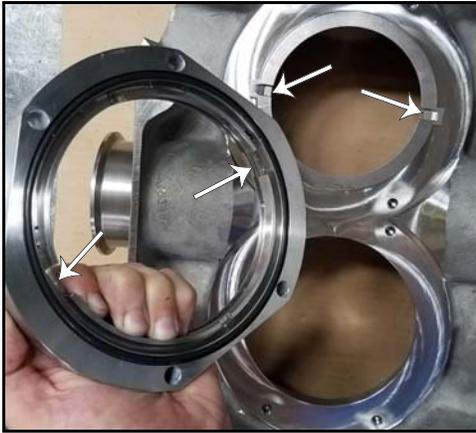
**Figure 110 - Seal housing O-ring installed**
