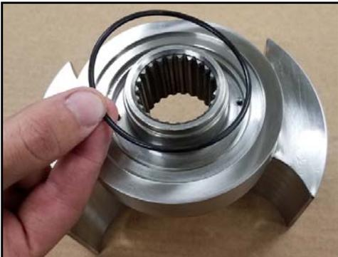
**Figure 169 - Install sleeve front O-ring**
