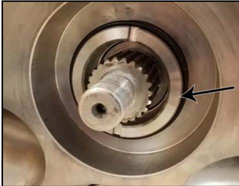
**Figure 141 - Sleeve remaining after rotor removal**
