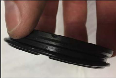
**Figure 131 - Seal O-ring installed**
