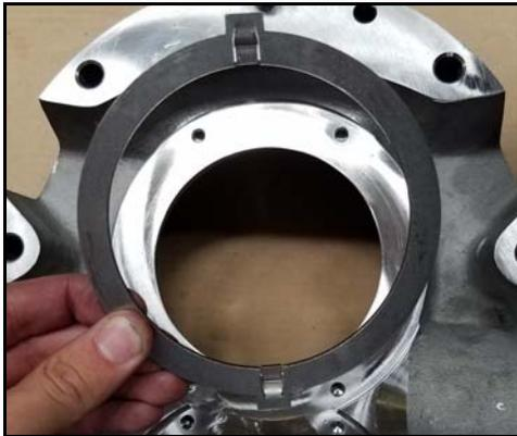
**Figure 60 - Install drive ring**
