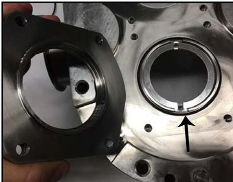
**Figure 75 - Remove seal housing**
