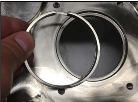
**Figure 79 - Remove shaft ring**
