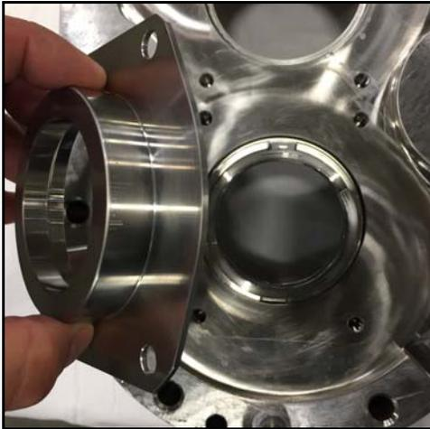
**Figure 57 - Install seal housing**
