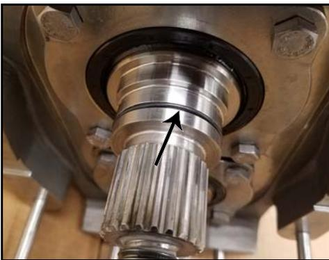
**Figure 161 - O-ring installed**
