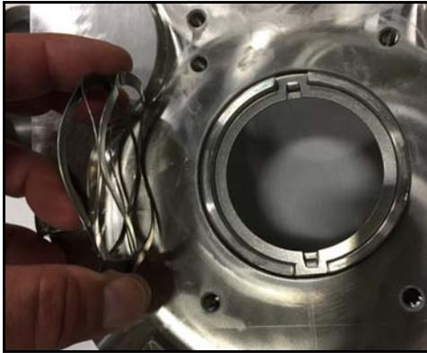
**Figure 47 - Remove wave spring**
