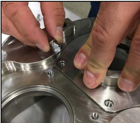
**Figure 58 - Install seal housing bolts**
