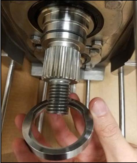
**Figure 153 - Remove seal seat**
