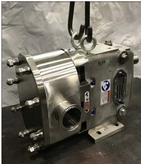
**Figure 3 - Lifting location**
