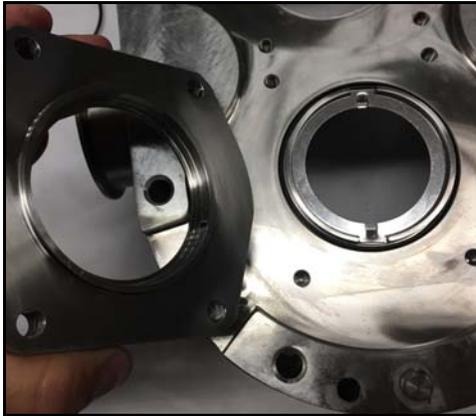
**Figure 87 - Install seal housing**
