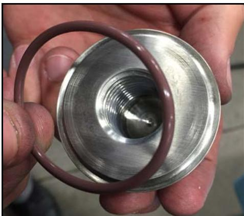
**Figure 179 - Install O-ring**
