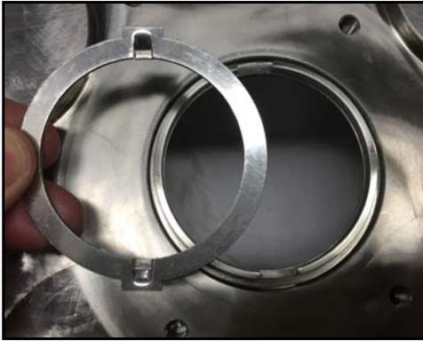
**Figure 83 - Install drive ring**
