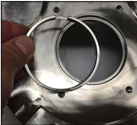
**Figure 49 - Remove shaft ring**
