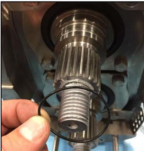
**Figure 99 - Install O-ring**
