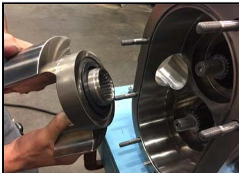
**Figure 37 - Remove rotor**
