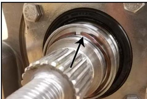
**Figure 152 - Remove wave spring**
