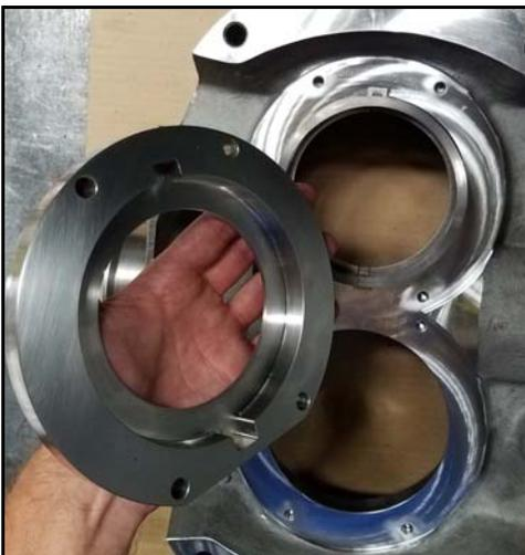
**Figure 46 - Remove seal housing**
