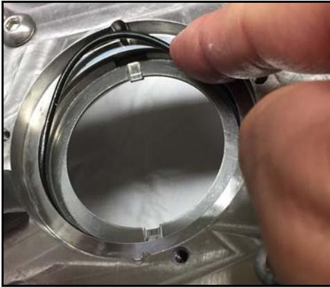
**Figure 90 - Install seal O-ring**
