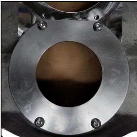
**Figure 65 - Seal housing installed**
