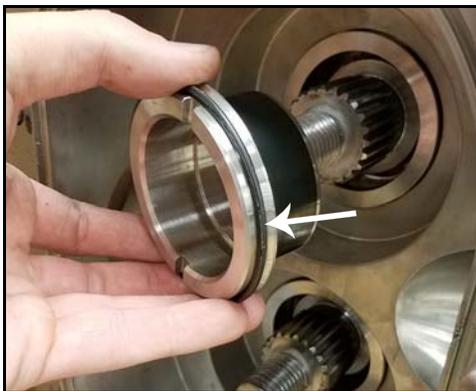
**Figure 142 - Remove sleeve, O-ring**
