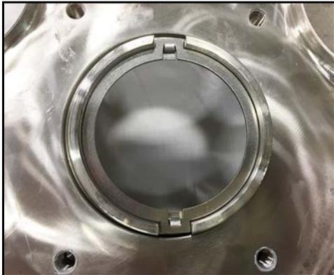
**Figure 54 - drive ring installed (130-U3 and smaller)**
