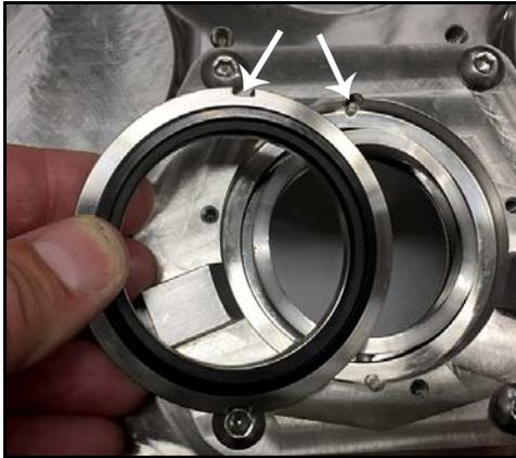
**Figure 94 - Install flush-side stationary seal**
