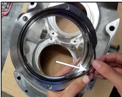
**Figure 109 - Install seal housing O-ring**
