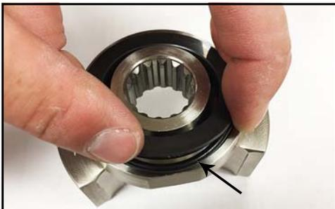
**Figure 139 - Seal O-ring pinched**
