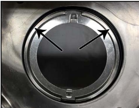
**Figure 86 - Seal housing O-ring installed**
