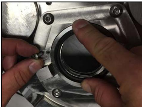
**Figure 96 - Install seal retaining bolts**
