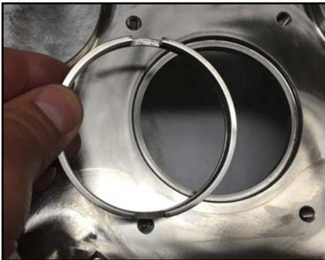
**Figure 51 - Install shaft ring**
