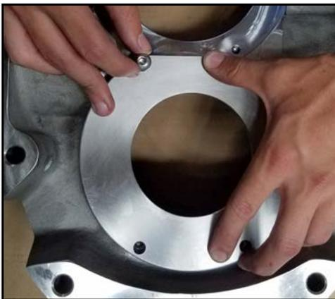
**Figure 64 - Install seal housing bolts**
