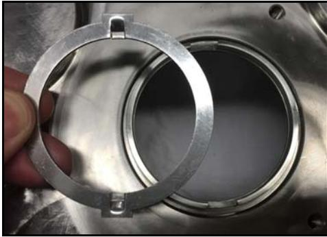
**Figure 53 - Install drive ring**
