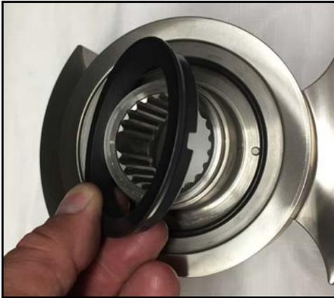
**Figure 137 - Install rotary seal**
