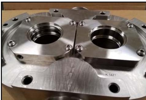
**Figure 159 - Seal housings installed**
