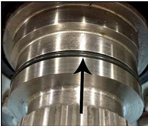
**Figure 120 - O-ring installed**
