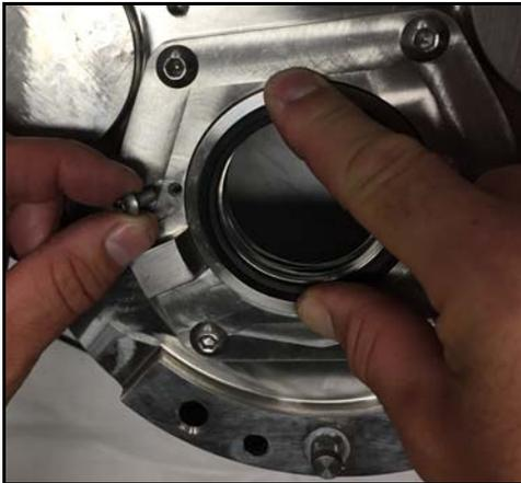
**Figure 70 - Remove seal retaining bolts**
