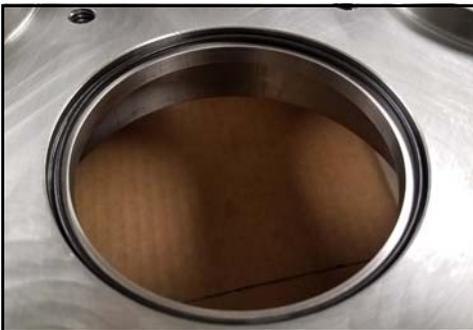
**Figure 155 - Seal housing O-ring installed**
