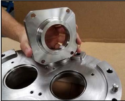
**Figure 156 - Line up bolt holes**
