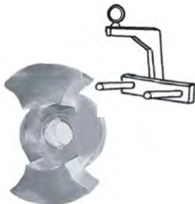
USE ROTOR REMOVAL TOOL TO REMOVE ROTORS
