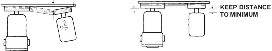
After piping is complete and before belts are installed, **turn pump shaft manually** to see that it turns freely. Check rotation direction of pump to see that pump will rotate in proper direction (see figure 1) Install belts and tension them correctly. Install belt guard.
