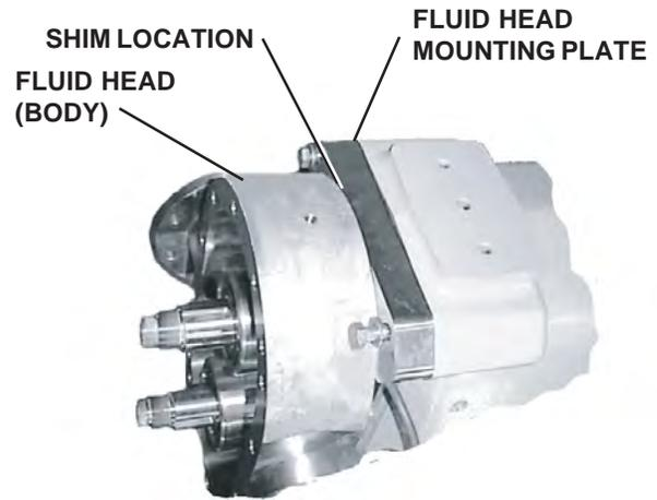
1. Install the pump fluid head on the gearcase. Make sure that all mating surfaces between the fluid head mounting plate and the gearcase mounting surface are clean and free of all burrs. The shaft seals need not be installed for this operation, and it is much simpler if they are not.
