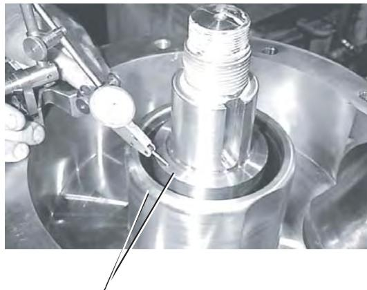
**MEASURE BOTH SHAFT S. APPLY SHIM UNDER FRONT BEARING SEAT, IF REQUIRED.**
