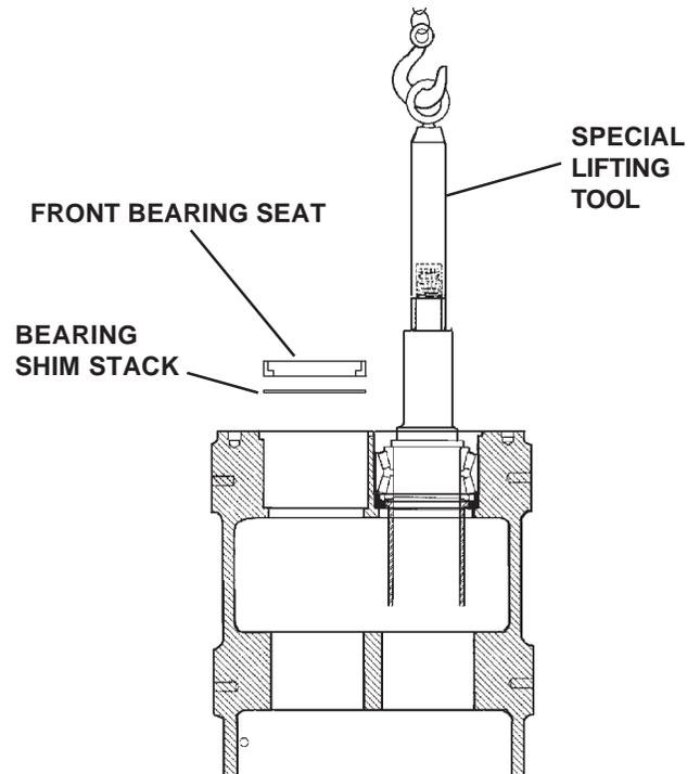
5. Before continuing, a critical measurement must be taken to determine the need for a bearing shim. measure the distance between the fluid head mounting surface and the rotor seat surface on the corresponding shaft. Do this for both shafts. If both dimensions are the same, then no shims are needed. If there is a difference, then a shim must be added to the shaft assemble with the shortest dimension. The thickness of the shim is equal to the difference between the two measurements.
