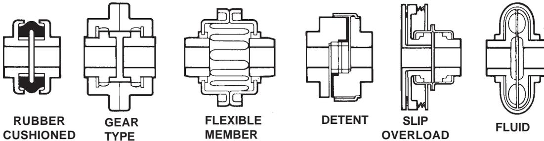
A flexible coupling is used to compensate for end play and small differences in alignment. The pump and drive shaft should be aligned as closely as is possible.
