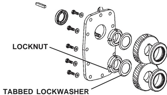
**(Note: The locknuts were installed with a minimum of 600 foot-pounds of torque using a special spanner type socket. A shaft locking device was also used to keep the shafts from rotating during the tightening operation.)**
