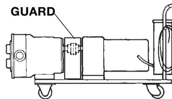
**Portable bases**-for movement to different locations. Many Commercial types are available.
