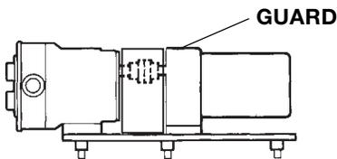
**Adjustable leg base**, commonly used for sanitary pumps. For washdown under base. Can be easily moved or repositioned.
