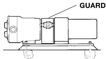
**Permanent** installation on foundation with bolts and grout. (Level unit before grouting.)
