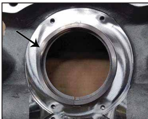
Figure 62 – Ressort ondulé installé
