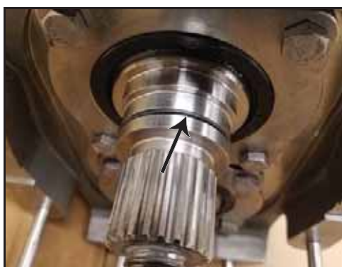
Figure 161 – Joint torique installé
