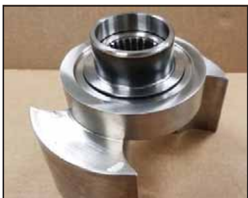
Figure 173 – Manchon de la garniture installé
