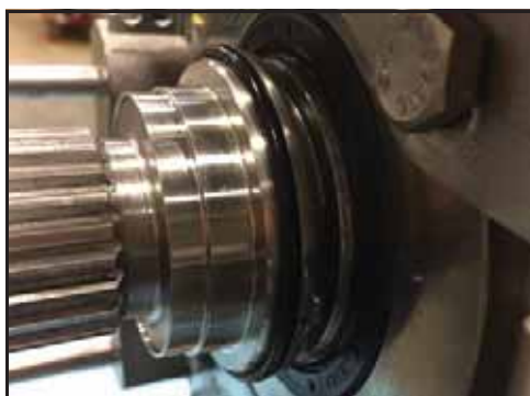
Figure 104 – Joint torique installé
