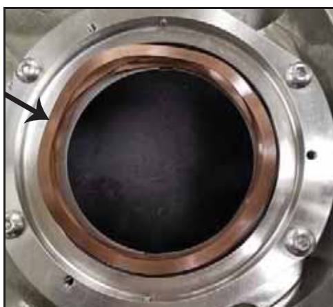
Figure 115 – Ressort ondulé installé
