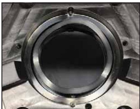
Figure 93 – Ressort ondulé installé
