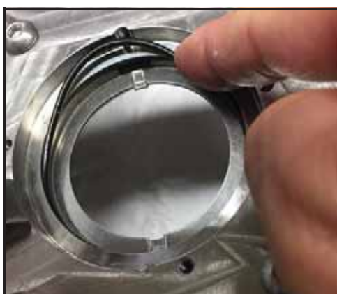
Figure 90 – Installation du joint torique de la garniture
