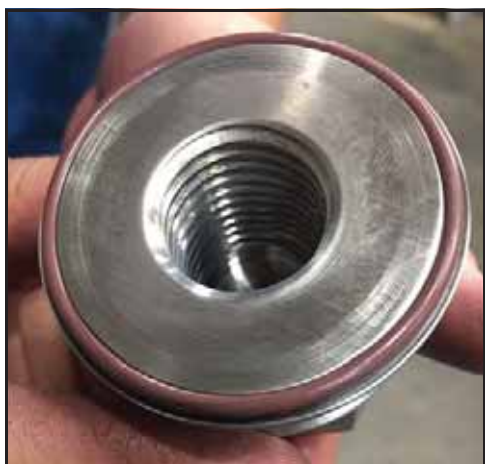
Figure 180 – Joint torique installé
