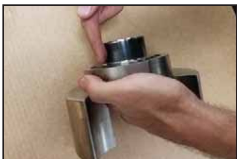
Figure 174 – Lubrification du manchon de la garniture
