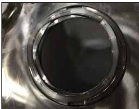
Figure 56 – Ressort ondulé installé
