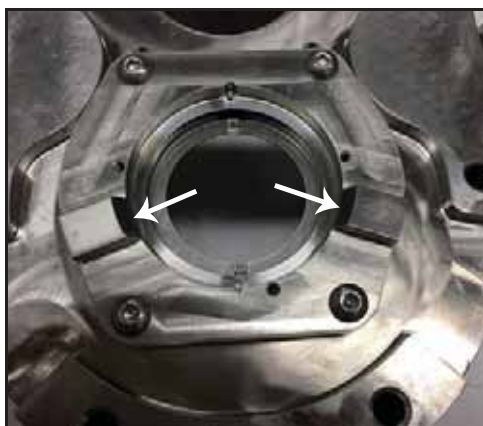
Figure 89 – Logement de garniture installé
