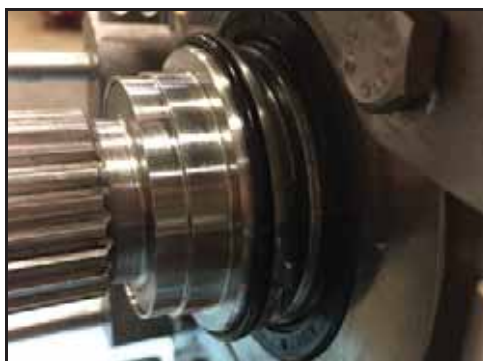
Figure 124 – Joint torique installé
