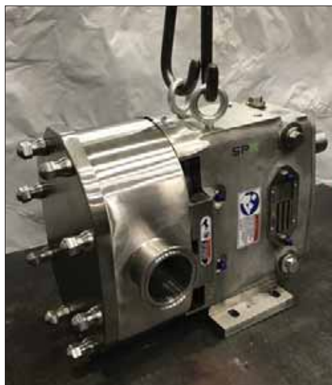
Figure 3 – Points de levage
