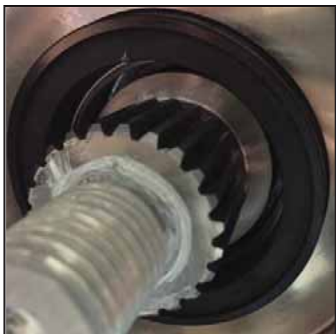
Figure 134 – Garniture fixe installée
