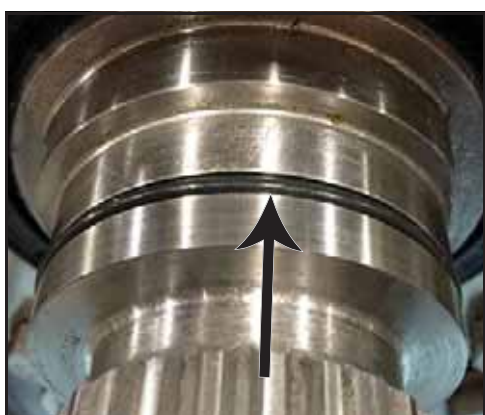
Figure 100 – Joint torique installé
