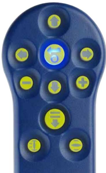
The Rotork *Bluetooth*® Setting Tool Pro with the relevant navigation and configuration keys is shown below.
