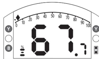
Fig. 4.4.4 Torque (A) + Position
