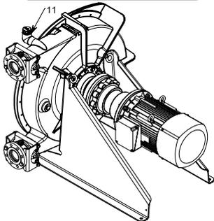
Fill the pump with corresponding volume of lubricant :
