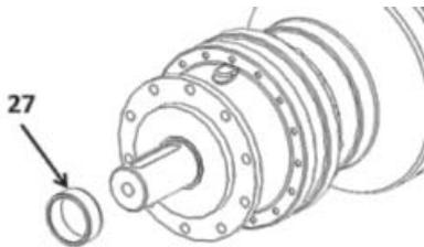
Heat new friction ring at  $110 \pm 10^\circ\text{C}$  /  $230 \pm 50^\circ\text{F}$ .
