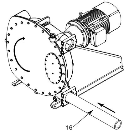
If pump rotates anti-clockwise, suction is on the top port :
