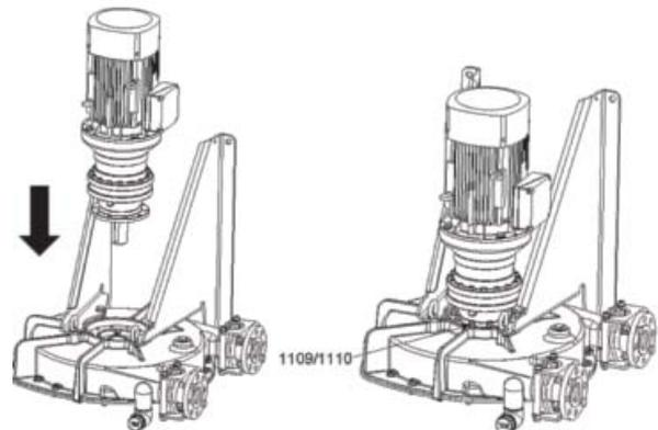
Put back studs 41 with their nuts 42 (HD50 - HD65) or screws 1109 with their washers 1110 (HDX65 - HDX80 - HD80) and tighten them.
