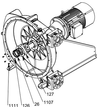
Refit rotor in the pump (see § ROTOR REMOVAL), refit hose (see § HOSE REPLACEMENT) and fill the pump with lubricant (see § LUBRICANT REPLACEMENT).
