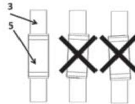
Rotate rotor and shoes assembly slowly and carefully check that no part comes in friction against pump body.
