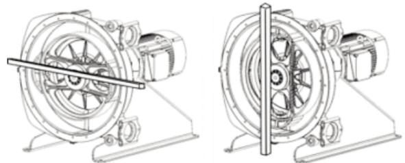
Put cover gasket 10 in pump body, starting at the top. Make sure that the two ends of gasket are firmly in contact.
