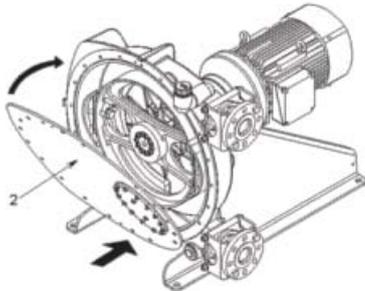
Screw and tighten screws 33 and their washers 34, starting by top ones to secure cover assembly.
