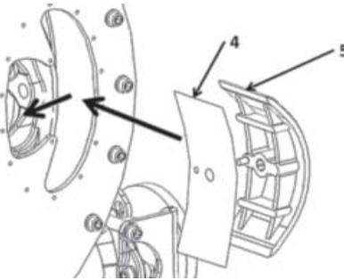
Check window seal 46 and replace it if necessary.
