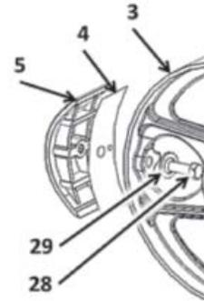
Screw and tighten screws 28 with their washers 29, carefully checking shoes 5 alignment with rotor 3.
