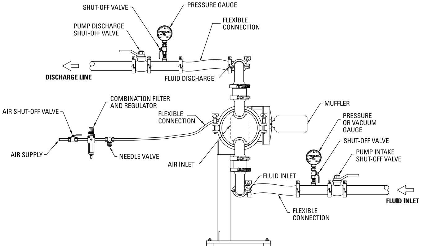
**NOTE:** In the event of a power failure, the air shut-off valve should be closed if restarting of the pump is not desirable once power is regained.
