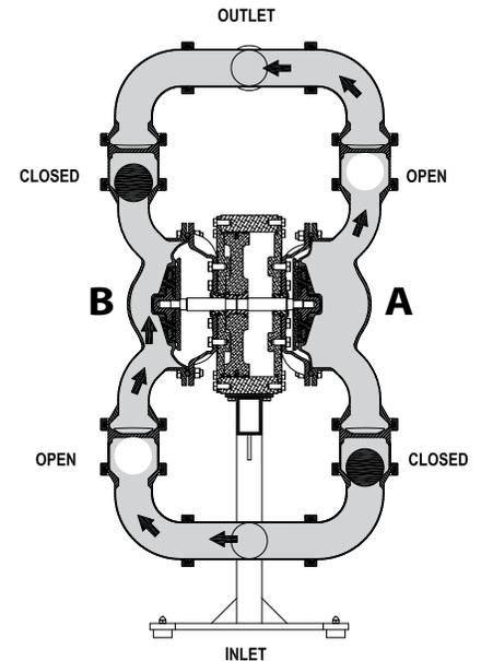
**FIGURE 3** At completion of the stroke, the air valve again redirects air to the back-side of diaphragm A, which starts diaphragm B on its exhaust stroke. As the pump reaches its original starting point, each diaphragm has gone through one exhaust and one discharge stroke. This constitutes one complete pumping cycle. The pump may take several cycles to completely prime depending on the condition of the application.
