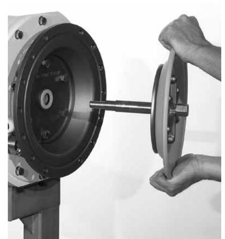
**AIR VALVE/CENTER-SECTION DISASSEMBLY**
