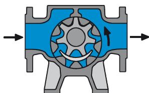
The rotor and idler gear mesh and liquid is being pushed into the discharge line.
