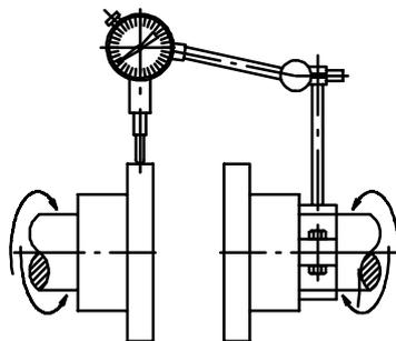
1. Fit the dial gauge to the drive shaft and check concentricity of both hubs by turning, if necessary realign.
