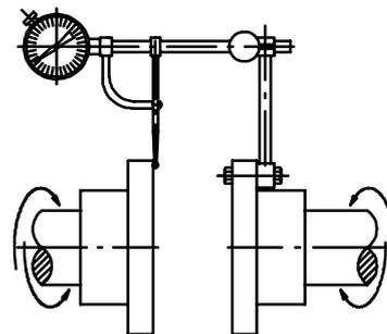
2. Fit the dial gauge to the flange of one hub and check the symmetry of both hubs by turning, if necessary realign.
