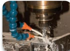
Machine Tool Coolant Feed
