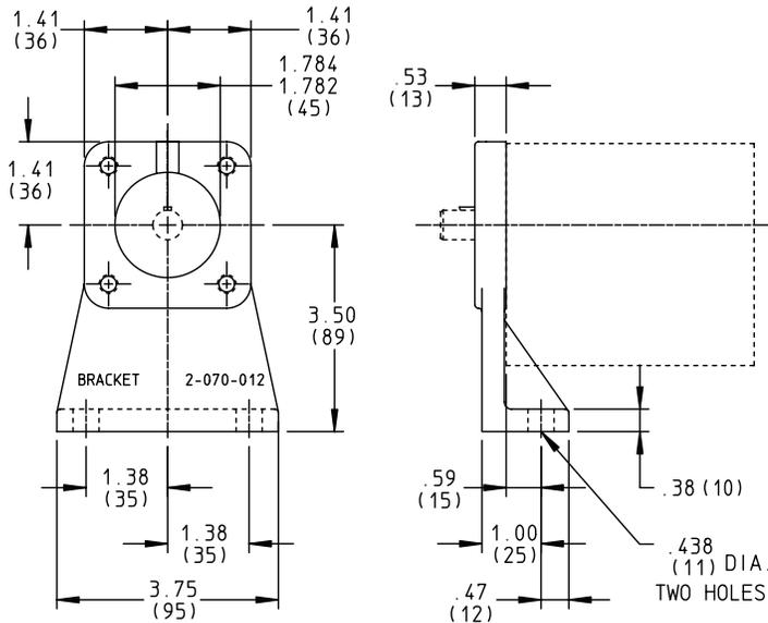
Note: Shaft height corresponds to Viking's "A" reducer or NEMA 56, 143T and 145T motors.
