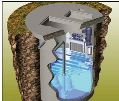
*Discreen / Muncher combination for pump protection*
