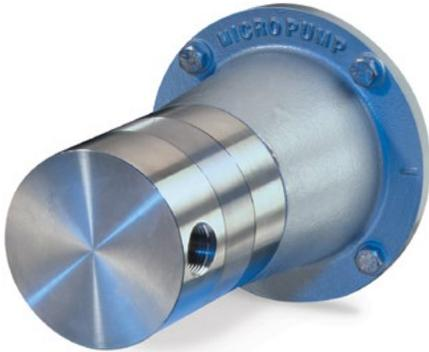
Series GN pumps deliver exceptional pumping performance for any high-precision application. These magnetically driven gear pumps feature a cavity style design with benefits such as chemical resistance, smooth pulseless fluid delivery, and high-system pressure capability. Available in standard and custom configurations, Micropump's Series GN pumps keep your operations running smoothly.
