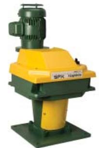
Our dry well construction removes the risk of lubrication leakage into the mixing chamber. The bearings are immersed in the gearbox lubrication which ensures that they continue to perform under high loads. Oil changes are made easy with our NEW tall pedestal which allows a 5 USGal. (20 liter) pail to be placed beneath the oil drain.
