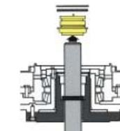
Seal changes are performed in less than 30 minutes. Simply loosen hardware and lower the shaft support collar onto the hub shoulder (1). Once the split coupling has been removed (2), lift off the seal assembly and replace with a new or rebuilt unit (3).
