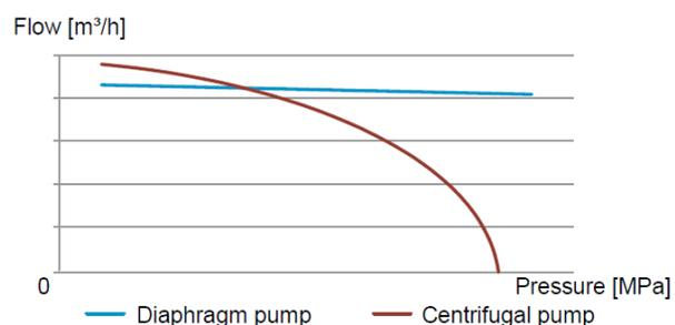
Flow vs. pressure operating curve
