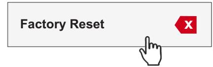
The Factory Reset dialog box will appear. Note that a Factory Reset will reset the device's configuration to default as well as clear all totalizer values from the device's memory.
