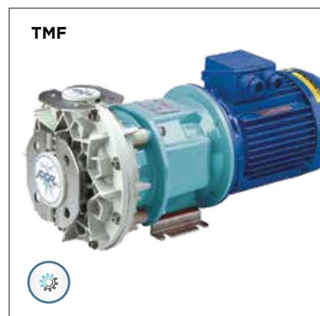
The pump casing is made of fluoropolymer with a nerve shape of 8-10mm thickness should be covered with an AISI 316 armour. These materials ensure the maximum protection level and chemical resistance.
