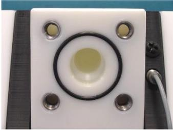
This version offers the possibility to use flange connectors according to DIN/PN 10 or ANSI. Thread bushings made of stainless steel (code F3/F4/F5/F6 respective F3w/F4w/F5w/F6w for ANSI) to fix the flanges are included in the center housing. The O-rings attached have to be inserted into the grooves of the manifolds to improve sealing before connecting the pump. The O-rings, flanges [30] are made of EPDM (code F 3), FEP (code F 4), NBR (code F 5) or FKM (code F 6).
