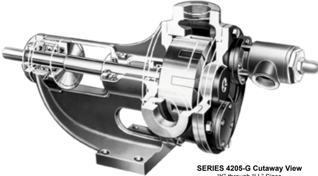
**SERIES 4205-G Cutaway View**
