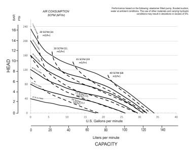
NOTE: Performance based on the following: elastomeric fitted pump, flooded suction, water at ambient conditions. The use of other materials and varying hydraulic conditions may result in deviations in excess of 5%.
