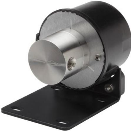
When you need a high-differential pressure, low-flow pump that delivers high performance in a small package, Series GAF is an excellent option. Series GAF gear pumps provide precise, pulseless flow, and features Micropump's suction shoe design. The suction shoe self-compensates for wear, ensuring near zero slip and long pump life. This pump, standard with an electromagnetic EagleDrive™, provides a highly efficient, compact pumping package that easily integrates into your design.
