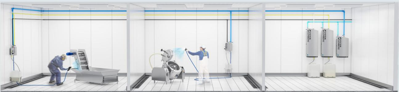
A hybrid solution has the same setup as a central system but with the additional possibility of adding an extra product at all or some of the workstations. The solution is often applied when there is a need for an extra cleaning task to be performed independently of the regular cleaning program.
