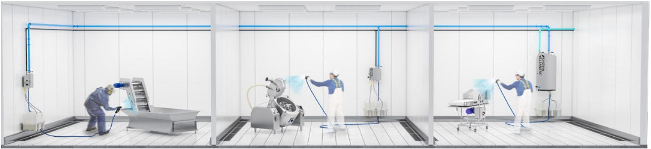
With a decentral solution, the concentrated chemicals are stored and dispensed at each workstation. This can be a main station or a satellite.
