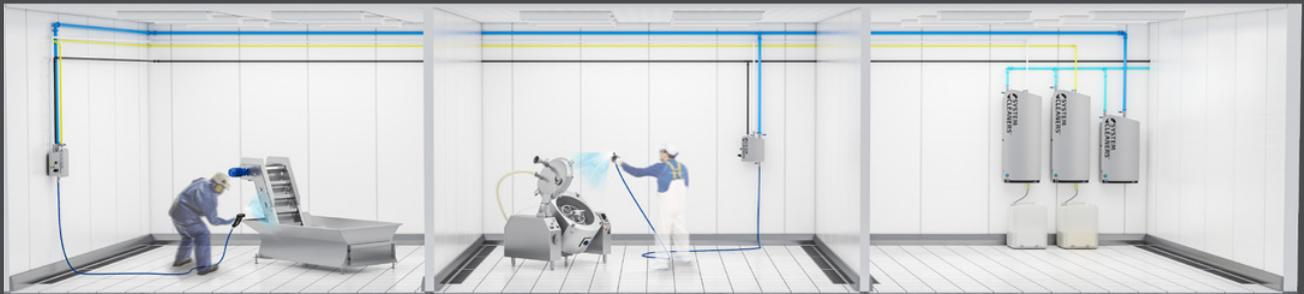
A central solution is characterized by prediluted chemicals being pumped to each workstation from a chemical pump station placed in a separate, central location.
